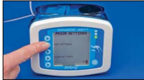
6) Power the pump on. Select "Keep Settings" to continue with previous setting or "Clear Settings" to start with programming new pump settings.
