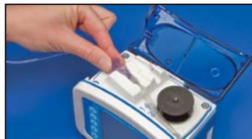
1) Grasp thumb tab on valve and insert into left pocket, ensure valve is fully seated. Thumb tab should align with slot in blue door.
