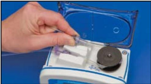
2) Grasp black ring retainer, gently wrap tubing around rotor, and insert retainer directly into right pocket. **Do not overstretch tubing.**
