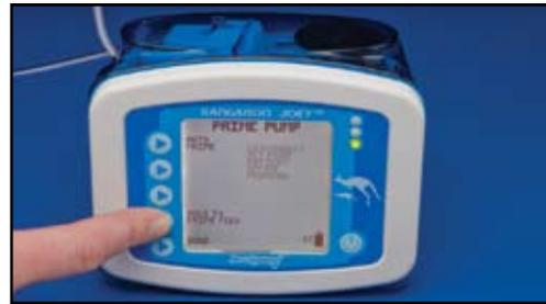
8) Press and hold the "Hold to Prime" button until only clean water flows through the tubing. Once the rotor starts this takes between 1 and 2 minutes.
