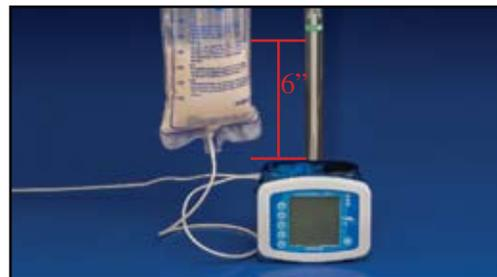
10) **CAUTION-** To achieve proper accuracy the fluid level in the feeding set bag must be 6" above the top of the feeding pump, when initiating the feeding cycle.
